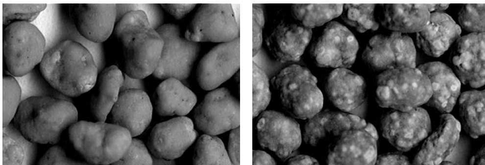
Figure 1. NPK 15-15-15, low abrasion capacity (left), and NPK 15-15-15, high abrasion capacity (right).
