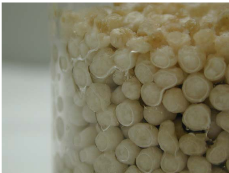
Figure 2. Detail of ammonium nitrate moisture absorption at laboratory scale in a climatic chamber.
