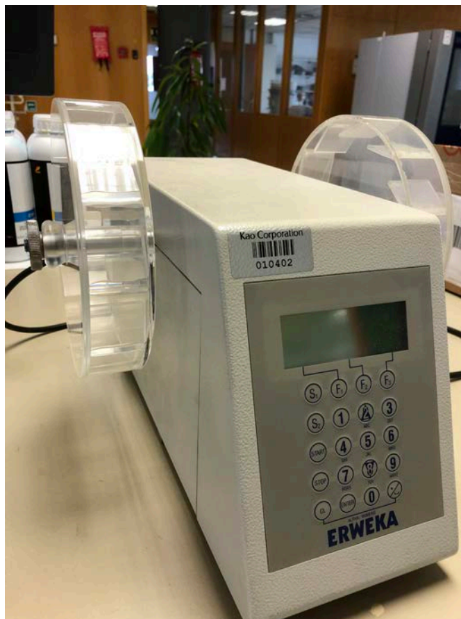
Figure 6. Rotary drum for abrasion test.
