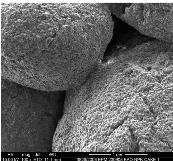
Figure 4. SEM images of two examples of crystal formation on a granule's surface, where the crystals have a needle shape that promotes dust formation.
