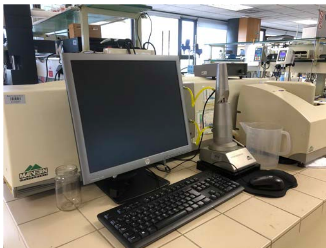
Figure 7. Mastersizer 2000 used to measure particle size distribution of the dust released from fertilizers.
